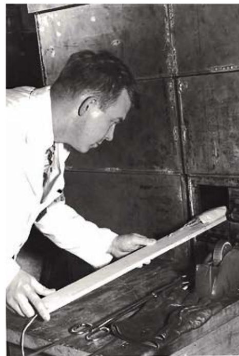
Elmer Rylander inserting corn tassels into the thermal column of CP-3 in 1946. The irradiated pollen was used in a research program conducted by Thad Pittenger at the University of Nebraska.
